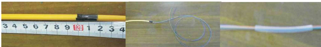
Pic3: the length of stripped fiber cable
