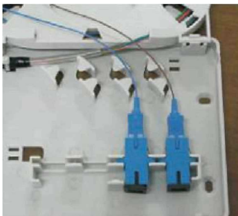
Pic11: install the adaptor and pigtail
