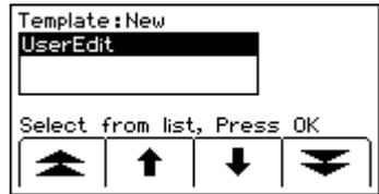
Step 7. Move the boxed cursor by pressing the left/right arrows [SK] or up/down arrow [SK] to move the cursor up or down.
