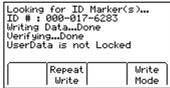
**Note:** Once the marker data has been locked, the information contained on the marker is **PERMANENT**. Choosing to permanently lock the marker data is irreversible. Once the data is locked it can not be overwritten. Assure that the data that is being written is correct before proceeding.
