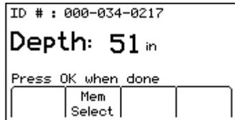
Step 3. To save the depth reading, press *Mem Select* [SK].
