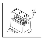
Press and hold OFF [T-1] to manually test the batteries. The display and audio will indicate one of the following levels: (OK w/solid tone = good; LO w/beeping tone = low; "--" w/no tone = replace)
