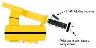
2. Slide battery compartment out of handle.
