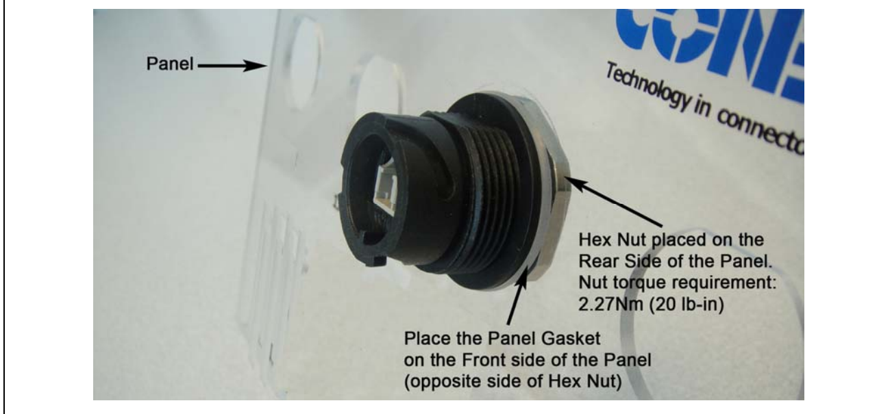
Figure 5-3: The Front Panel mount
