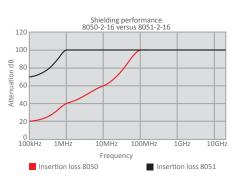
The 8050 series Power line filters for shielded cabinets is a superior filter housed in a two compartment casing that achieves 100 dB insertion transmission loss at 14 kHz till 40 GHz. The circuit is designed as a double- circuit with high quality rod cores providing inductance. These cores do not saturate due to their large air gap and they are insensitive to asymmetrical load.
